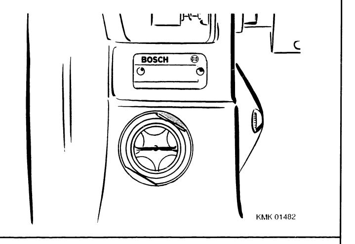
Move control rod of driving device in direction of dial indicator until adjusting pin can be inserted into recess in control rod.
